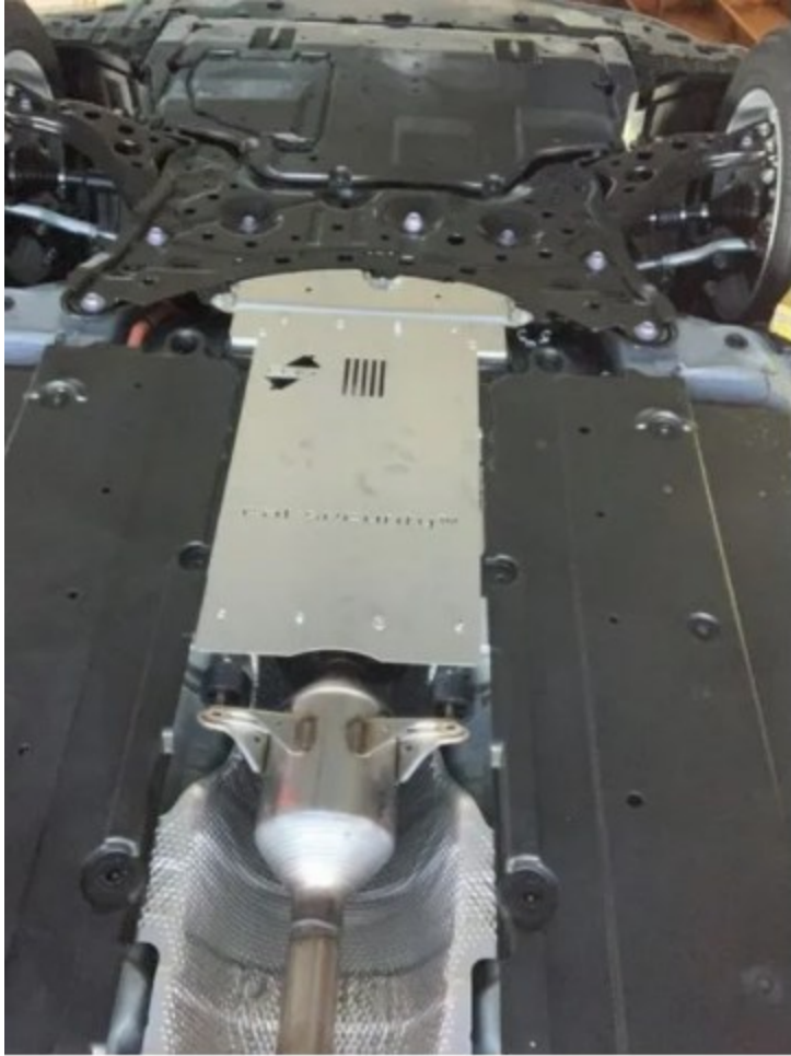
Catalytic Converter (cat shield for Toyota Prius and Honda Element)
